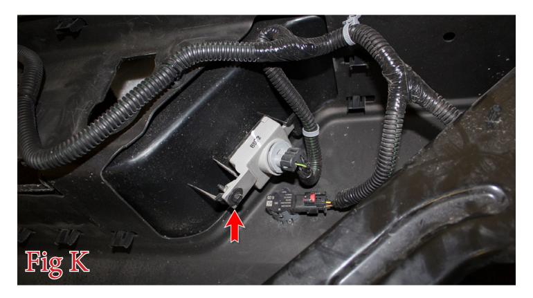
13. Unplug and remove the parking sensors. Do this by spreading the two tabs on the back side of the sensor mounting rings. Be sure to keep track of what position/orientation they are all installed on the OEM bumper so you can install them in the same position/orientation in your new bumper. (Fig L)
