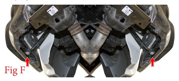
8. Using an 18mm Socket, remove the two mounting nuts (per side) that hold on the OEM bumper. Then, remove the OEM bumper from the vehicle. (Fig G)
