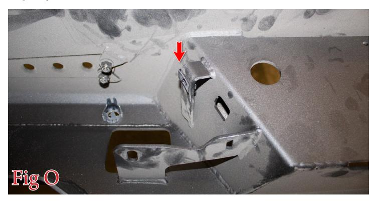
17. Set the license plate lights in place on your new bumper. The license plate lights will have to be switched, so the left light goes on the right side of the bumper and the right light goes on the left side of the bumper. Put the tab in place in the slot and use the supplied 1/4" Bolts (1 per side) and 1/4" Washers (1 per side) to hold the lights to the bumper. (Fig P) **DO NOT OVERTIGHTEN THESE BOLTS, ONLY TIGHTEN UNTIL THE LIGHT IS BARELY SNUG.**
