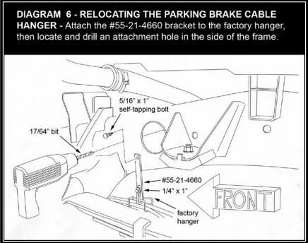
with the supplied 5/16" x 1" self-tapping bolt (13), then tighten the 1/4" bolt (76 in-lb.).
