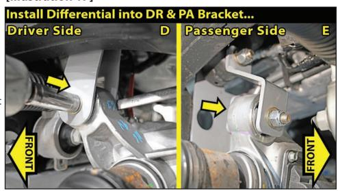
run the bolt from rear-to-front through the diff drop bracket, differential and support bracket. Attach with washer and Nyloc nut. Do not tighten at this time. [13/16" | 7/8"]
