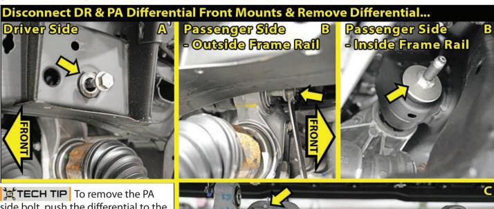
TECH TIP To remove the PA side bolt, push the differential to the PA side slightly and roll the back of the differential upward.
