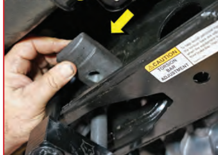
Illustration 56 Reinstall Retainer Block, Adjuster Bolt & Load Torsion Bar Passenger Side
