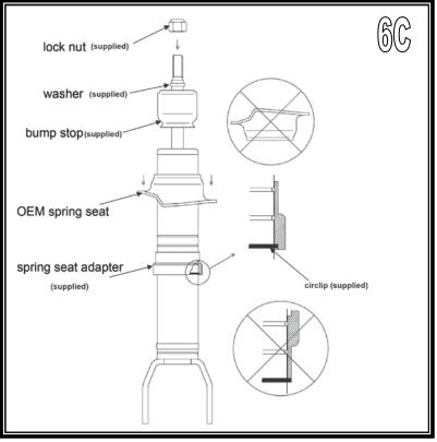
the appropriate groove. (4" kits typically use the bottom groove.) Remove the new bump stop from the Bilstein strut shaft.
