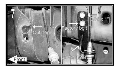
notch in the frame to allow removal of the brake hose / line connector. *Take care NOT to damage the brake line / hose.* Remove the brake line bracket bolt then free the line / hose connector from frame.
