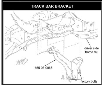
two recesses in the bracket that align with two existing frame rivets. Also note that the bracket's inside edge is contoured to match a similar edge on the frame. Align the two contoured edges, then using the bracket as a template, mark the location for two mounting holes to be drilled.
