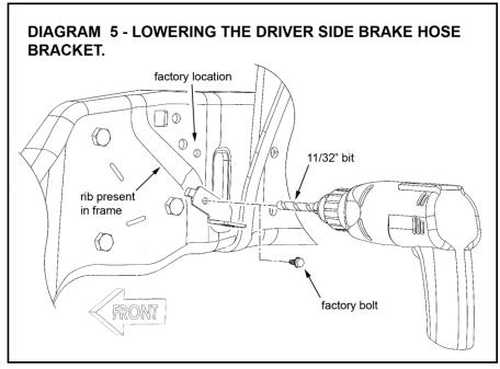
this location. Carefully reform the metal brake line so that the alignment tab in the brake hose bracket engages the existing hole in the frame as shown. Using the bracket as a template, mark the location of the second hole to be drilled.
