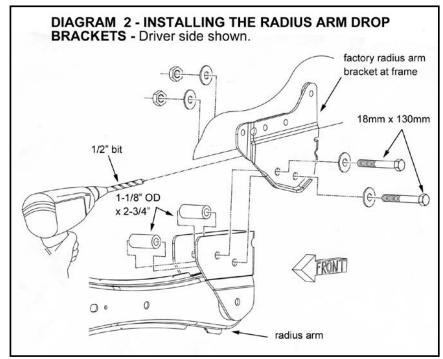
130mm bolts with washers through the factory mount, drop bracket, and sleeves. The bolts should be installed from the outside and secured with the remaining 18mm washers and nyloc nuts.
