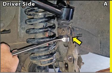
**15. REATTACH BRAKE LINE BRACKET TO KNUCKLE...** [Illustration 14] [] [Illustration 14] To allow additional slack in the line, remove the ABS line from the ABS/brake line bracket at the upper mount tab. Carefully bend the tab open with a flat screw driver taking care not to damage the ABS line.
