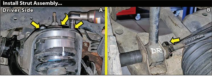
**14. CONNECT UPPER BALL JOINT TO KNUCKLE & TIE ROD TO KNUCKLE...** [] [Illustration 13-A] Connect the upper ball joint to the knuckle with the supplied castle nut. [13/16"] (81)
