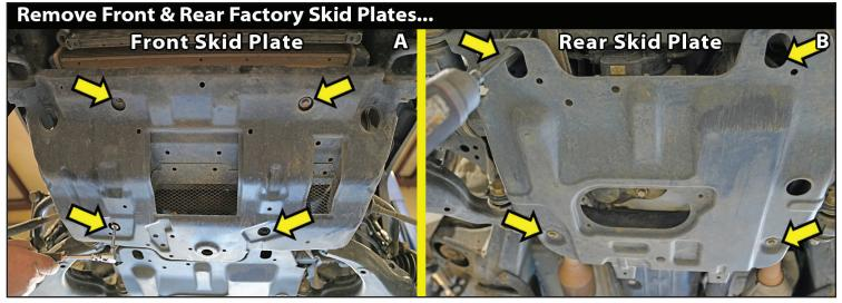
**TECH TIP** When you remove a factory nut or bolt, like the skid plate fasteners, sway bar links, ball joint nut, etc., put it back into the factory spot for safe keeping. You will not have to look or sort through removed hardware to find the proper factory fastener.
