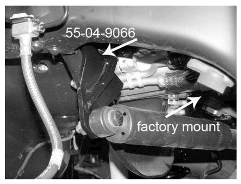
□□ A bracket attaches the brake line / hose assembly to the outboard face of the frame rail, just forward of the coil spring tower. Unbolt this bracket from the frame.
