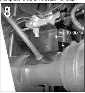
are clean and free of debris, then seat the pin in the block in the spring perch. Line up the center pin of the spring with the hole in the block, then raise the axle enough to seat the block.
